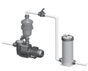
Typical installation with a sand filter
