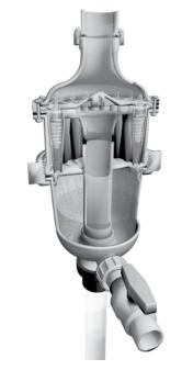
Incoming water is guided by a diverter plate so that it enters multiple hydro cyclones tangentially generating a strong centrifugal effect. This spins the sediment out to the hydro cyclone's wall and then spirals it down to the sediment chamber, while the cleansed water spirals upwards.
