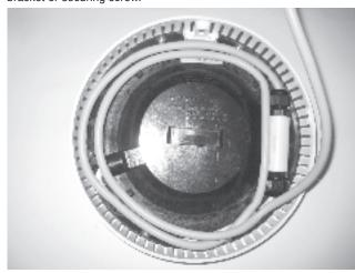
The light can now be switched on to check operation. Note that for Halogen light it should not be switched back on for at least 2 minutes after switching off to prevent blowing of globe.
