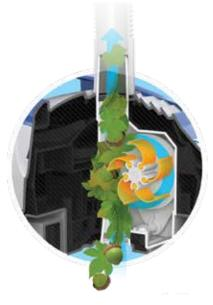
Patented anti-blocking design – features V-Flex<sup>™</sup> technology that virtually eliminates blockages
