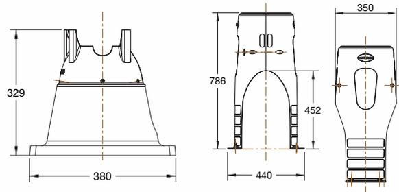
*Note: MultiCyclone Support Stand is suitable for most Waterco Domestic Pool Pumps. Excluding Hydrostar & all Commercial Pumps.*
